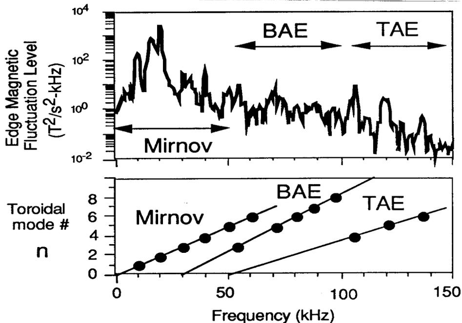
Fig. 4 - Edge magnetic fluctuation spectrum showing TAE modes driven by NBI in DIII-D. The TAE (and BAE) have mode numbers in the range  $n \approx 3-8$ . The TAE modes in ITER are expected to be unstable over the range  $n=5-50$ , implying a more complex frequency spectrum in ITER (figure courtesy of W. Heidbrink).
