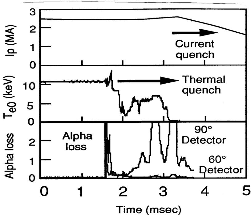
Fig. 3 - Measurement of DT alpha particle loss during a major disruption in TFTR. The disruption at 1.5 msec causes a rapid loss of  $\geq 10\%$  of the confined alphas before the current quench, mostly to the  $90^\circ$  detector. The loss at  $\leq 1.5$  msec is the normal first-orbit loss level.
