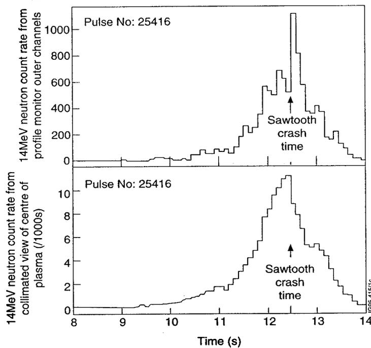
Fig. 2 - Measurements of triton burnup in JET showing a weak redistribution of confined tritons during a sawtooth crash. The top trace shows an increase in tritons near the plasma edge, and the bottom trace shows an decrease in tritons nearer the plasma center.
