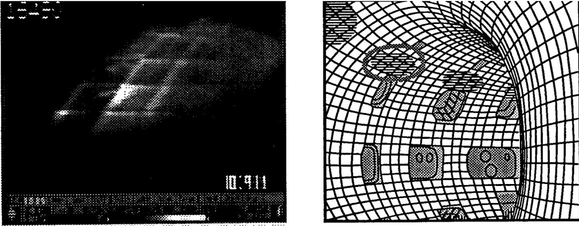
Fig. 1 - At the left is an IRTV image of the surface temperature of the JT-60U wall showing TF ripple loss of beam ions during perpendicular NBI. These hot spots occur just above the outer midplane between the TF coils (right). The heat flux in this case is  $\approx 1 \text{ MW/m}^2$ , similar to that expected for alpha ripple loss in ITER.
