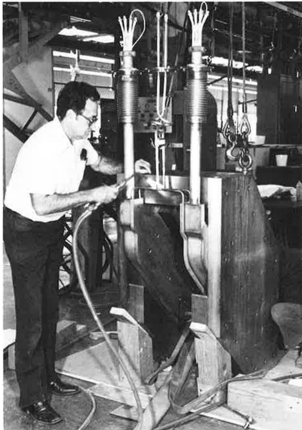
Figure 43. Final assembly of the PDX neutral beam deflection magnet.
