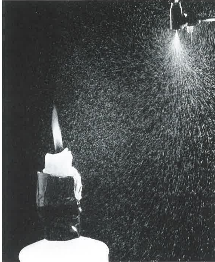
The design of novel fire sprinklers is just one of the many applications in the field of electrostatic atomization. The photo shows electrically charged water mist attracted to the flame of a candle. Being able to focus the water at the fire source eliminates the need to deluge an entire area thus preventing unnecessary water damage to materials not directly involved in the fire.
