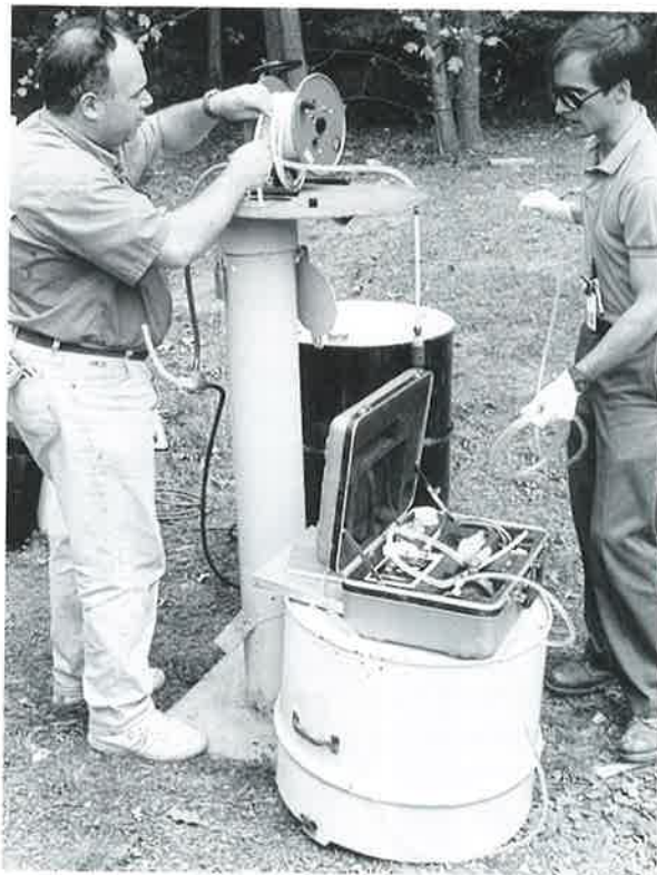
Environmental Restoration and Waste Management personnel measure groundwater level and prepare to collect samples using the new groundwater sampling system.
