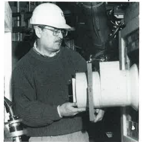
Imaging tube for the hard X-ray "pinhole" camera being inserted into shielding assembly. The lens and optical conduit for coupling the tube output to the image processing computer can be seen on the lower left side of the picture.
