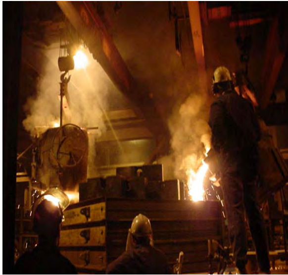
Figure 5. Pouring of a Casting
