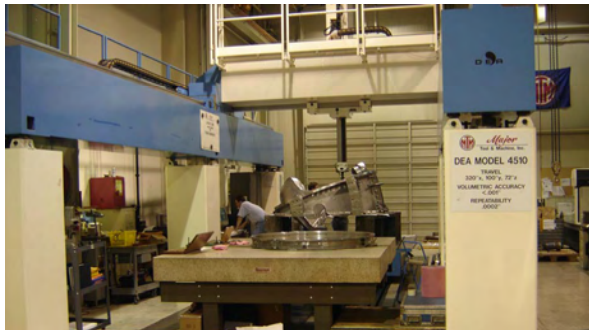
Figure 9. CMM Measurement of the C1 Winding Form
