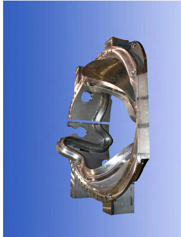
Figure 10. Photo of the C1 Winding Form
