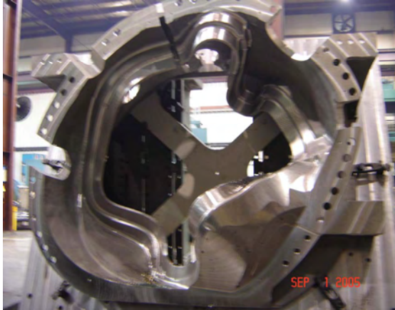
Figure 8. A Casting During 3-Axis CNC Machining
