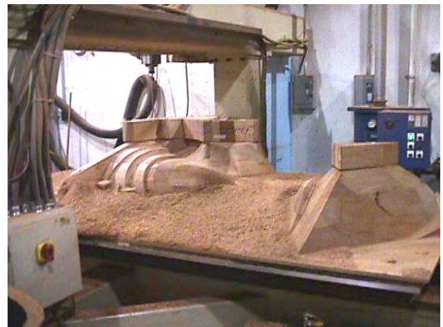
Figure 4. Contour Milling of a Pattern
