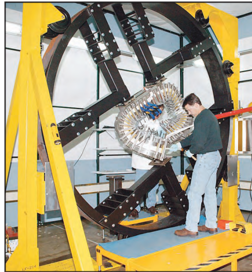
Figure 6. The Twisted Racetrack Coil in the vertical turning fixture which will be used for the winding of NCSX modular field coils.
