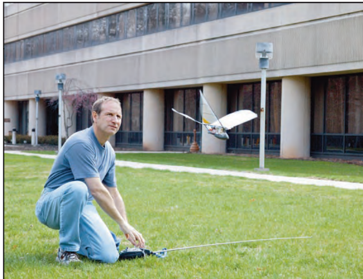
Figure 1. Dave Cylinder tests the ornithopter at PPPL. The ornithopter is a micro-air vehicle being developed in collaboration with the Naval Research Laboratory under the Survivable Autonomous Mobil Platform, Long Endurance (SAMPLE) Project. Micro-air vehicles generally have a wingspan of less than two feet and weight less than a pound. These aircraft are expected to perform useful surveillance missions.
