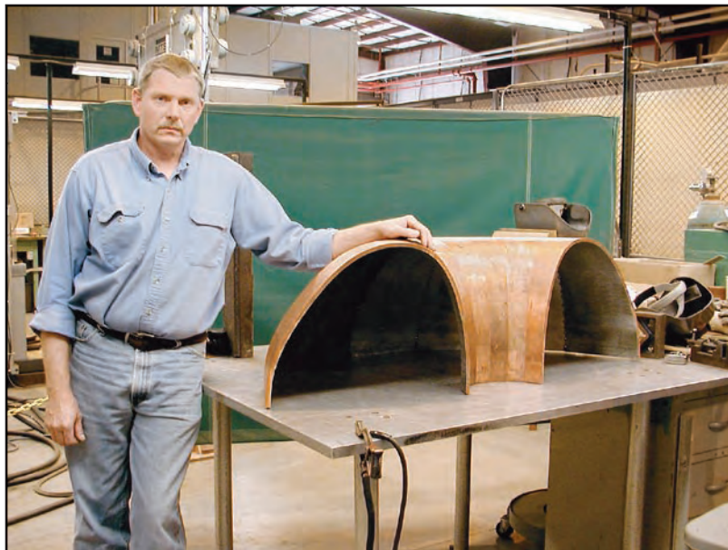
Figure 5. Conducting shell quadrant welded together by S. Jurczynski (pictured) of PPPL.
