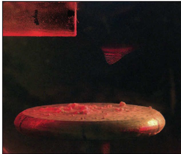
A dust cloud of silica microspheres is illuminated by laser light and suspended in a plasma. The dust cloud is approximately 0.5 inches high and floats in a conical shape between the dust tray and an electrode as long as the plasma is maintained. Fundamental dust cloud properties and dynamics have applications ranging from plasma processing to space plasmas.
