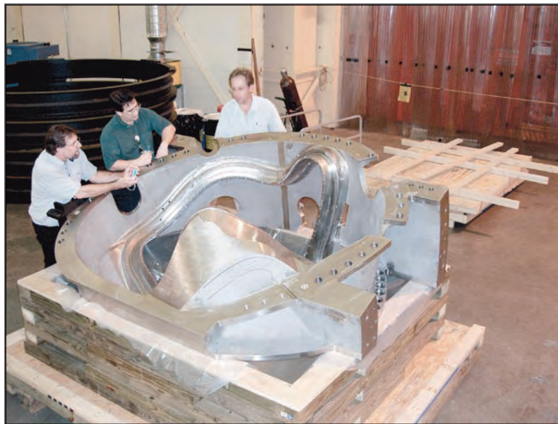
Figure 3. The first NCSX modular coil winding form is scheduled for shipment to PPPL in October 2005.
