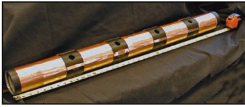
Figure 13. The one-meter-long ferroelectric plasma source is comprised of five shorter sources connected together, leaving space for diagnostic access.
