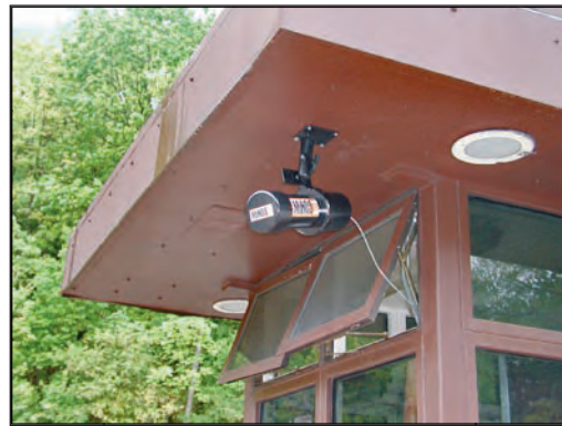
Figure 7. PPPL's Miniature Integrated Nuclear Detection System (MINDS) deployed at a facility entrance.
