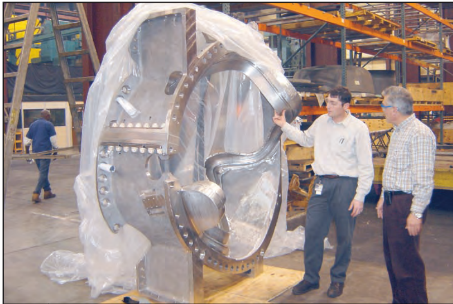
Figure 3. Finished modular winding form at the supplier's facility, ready to ship.
