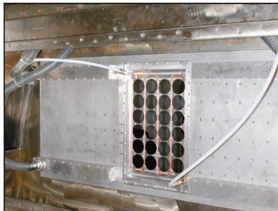
Figure 2. Anode insert with 24 hibachi windows installed for testing at NRL's Electra Laser Facility. The 24 round objects are the silicon wafers. The copper tubes provide edge cooling so when the electrons pass through the windows heat can be removed from the edges of the frame.
