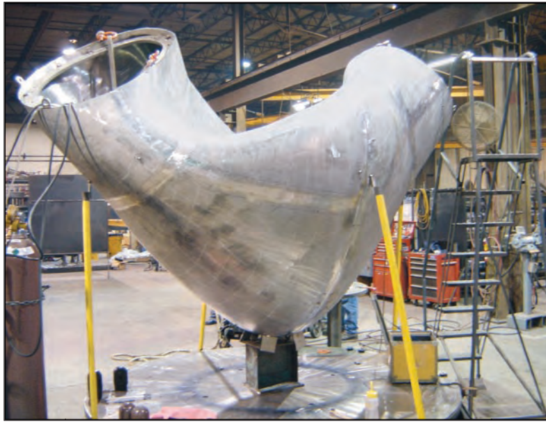
Figure 4. The first vacuum vessel subassembly in manufacture at Major Tool and Machine, Inc.
