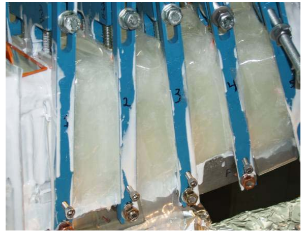
Figure 12 – Epoxy Shell Mold
