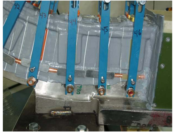
Figure 11 -VPI Bag under Vacuum
