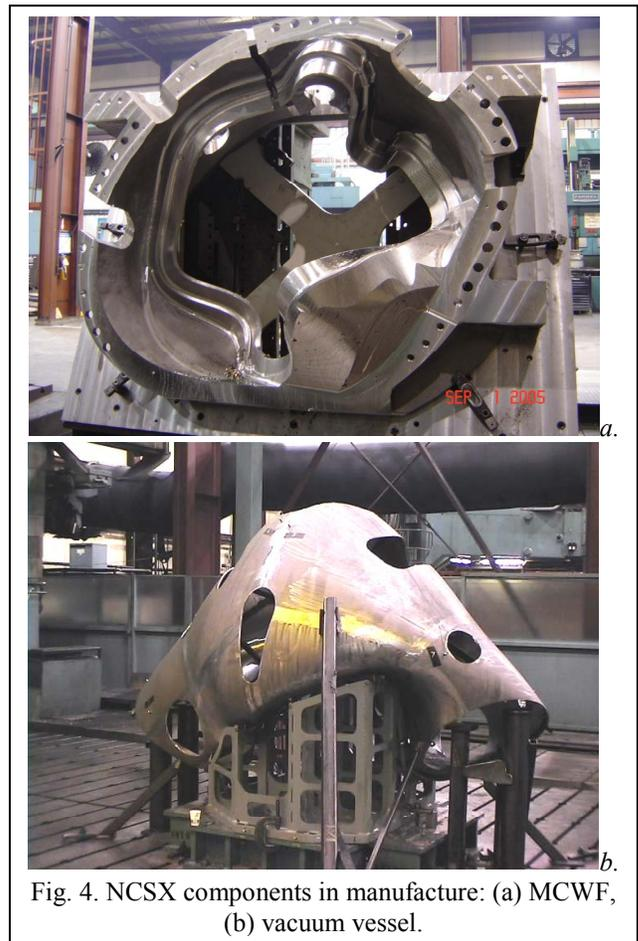
Fig. 4. NCSX components in manufacture: (a) MCWF, (b) vacuum vessel.
