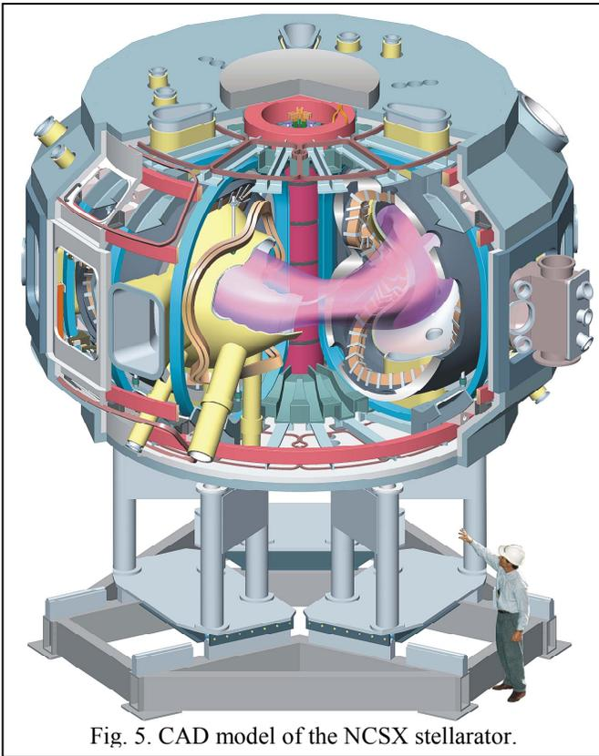
Fig. 5. CAD model of the NCSX stellarator.
