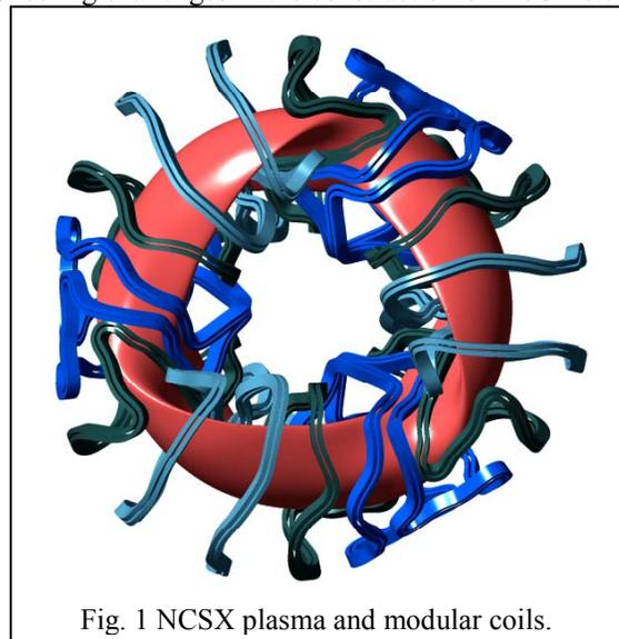
Fig. 1 NCSX plasma and modular coils.
