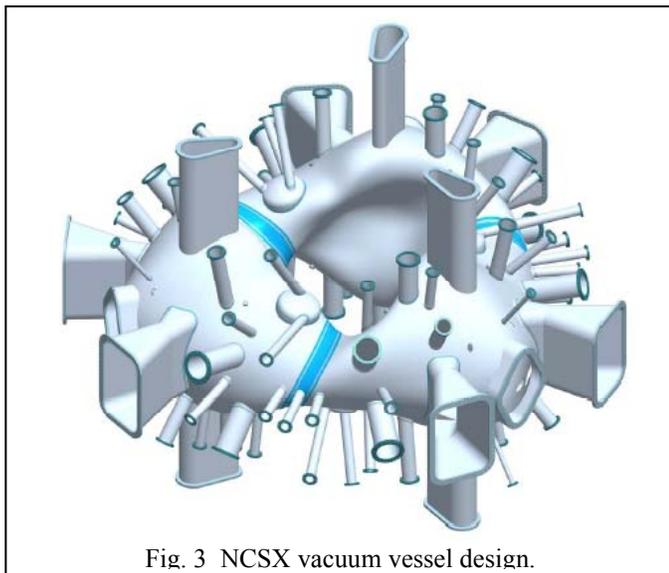
Fig. 3 NCSX vacuum vessel design.
