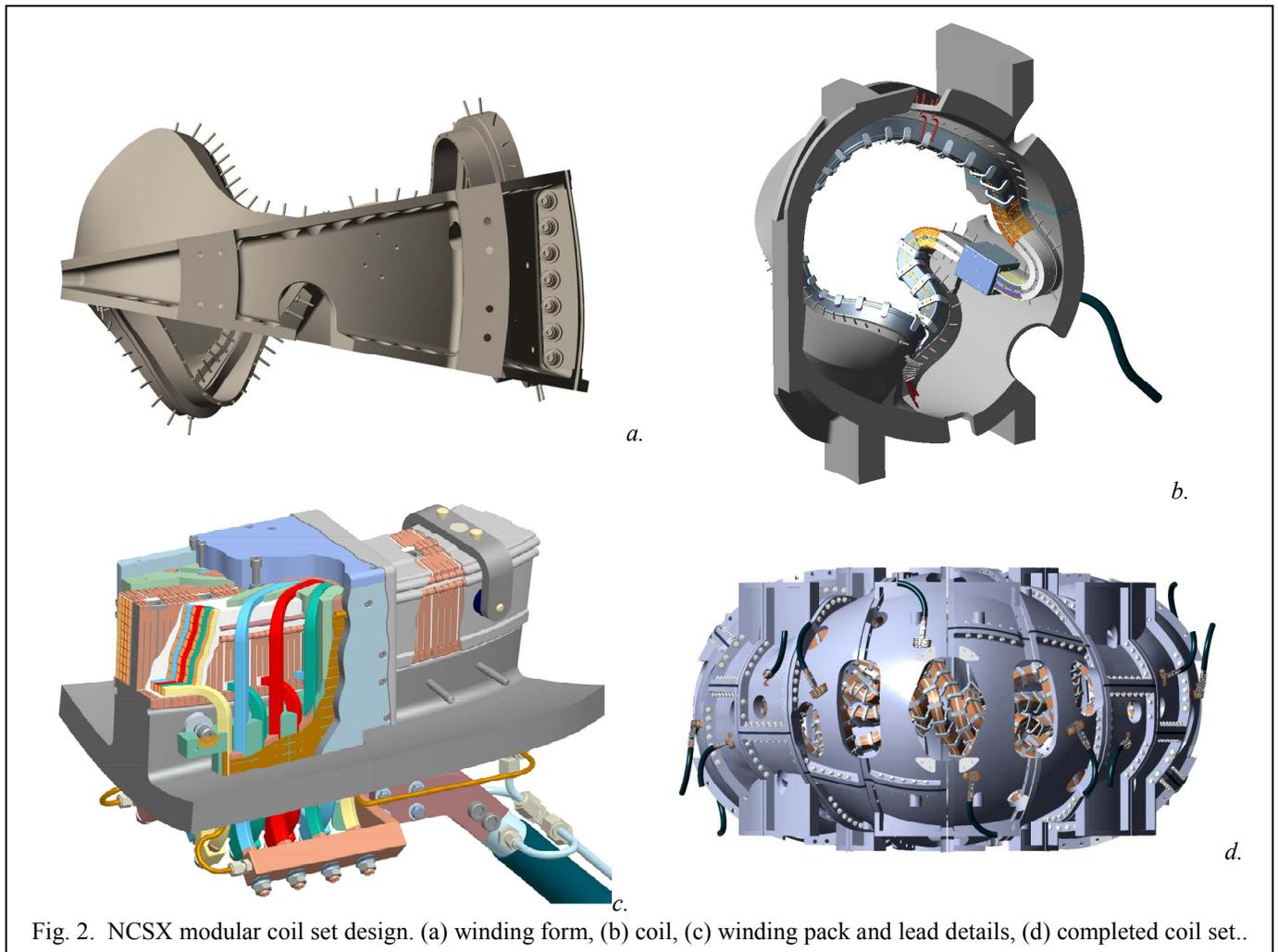
Fig. 2. NCSX modular coil set design. (a) winding form, (b) coil, (c) winding pack and lead details, (d) completed coil set..
