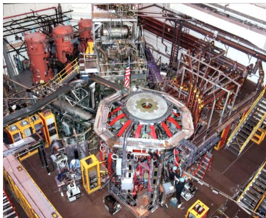
Fig. 1. An aerial view of the NSTX Test Cell. The NSTX device is in the center. The NBI beam box is located in the far side and the HHFW transmission lines to the right..
