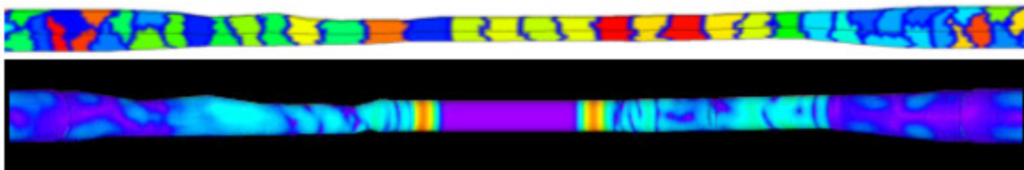
Figure 31. (Top) Distributed mesh of the IR between the crotches only. (Bottom) Snapshot in time of electric field due to two colliding beams from Tau3P time-domain simulation.
