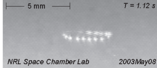
FIGURE 3. Direct laboratory observation of charged particle gyro-motion in magnetic field. [1]. (Reprint permitted by AIP and Dr. Amatucci.)
