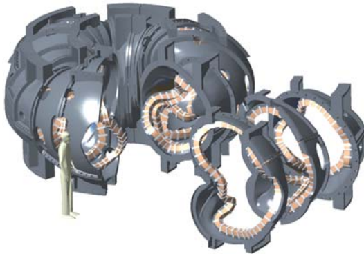
Figure 5. NCSX Modular Coil Structure
