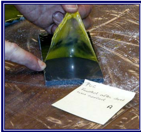
Fig 3. The thin films are removed after they have cured
