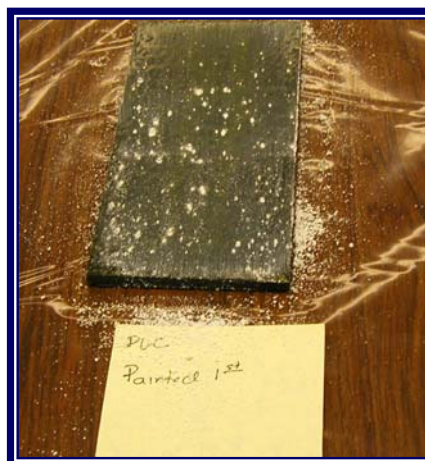
Fig 1. Luminescent dust is applied to the samples
