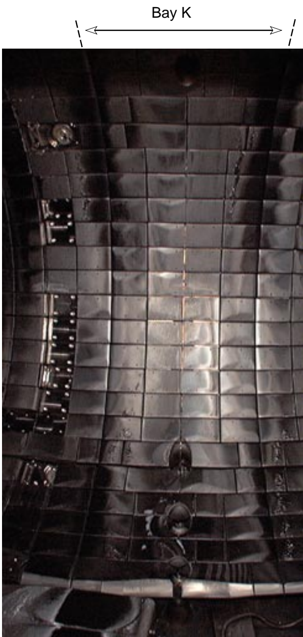
Fig.1 TFTR bumper limiter at Bay K on 17 th February 1999 showing co-deposition, flaking and white deposits. Some tiles have been removed from Bay L on the left. Deposition on a poloidal limiter tile may be seen at the lower left. The tiles are numbered by row from 1 (bottom) to 24 (top) and by column left (A) to right (D). The diagram depicts the tritium released (in Curies) from baking selected Bay K tiles (in parentheses Bay L tiles). Unshaded tiles are AXF-5Q graphite, gray shading denotes carbon fiber composite.
