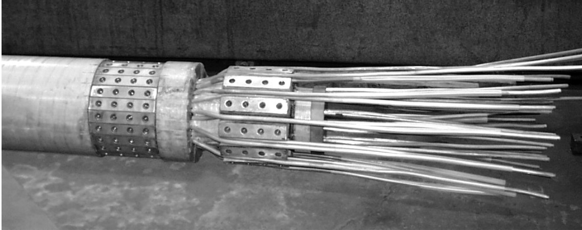
Figure 4 – End of TF Inner Leg Bundle After Fabrication, Prior to Assembly Showing Inner and Outer Leg Conductors and Water Cooling Tubes
