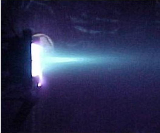
Fig. 8. Hall thruster operation
