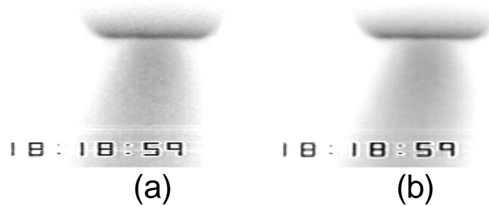
Figure B.3: Magnified view of the cathode region during instability in axial applied magnetic field shows no cathode spot motion. (a) a single frame with 10 \mu\text{sec} exposure. (b) the average of 30 consecutive frames, including the one shown in (a), taken over 0.5 sec. The average is almost identical to the single frame, indicating that the section of arc in the cathode region (and therefore, the cathode spot) was stationary during the instability. The waveforms corresponding to these 30 frames are given in Figure B.2. The axial magnetic field is 29 Gauss, average arc current is 254 A, electrode gap is 3.9 cm, frequency of column oscillation is 1190 Hz, the cathode used is #3 in Table 4.1. The horizontal scale is expanded 2.3:1.
