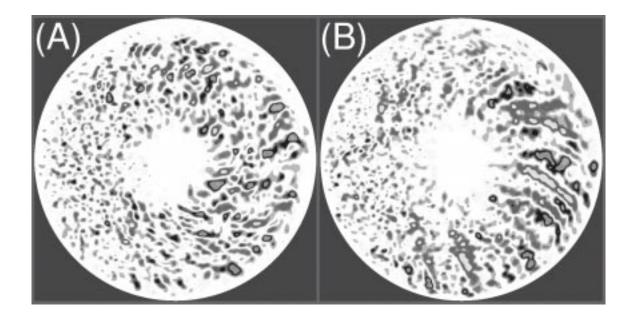
FIG. 1. Poloidal contour plots of fluctuation potential  $(e\Phi/T_i)$  in the steady state of a nonlinear global simulation with  $\mathbf{E} \times \mathbf{B}$  flows included (A) and with the flows suppressed (B).
