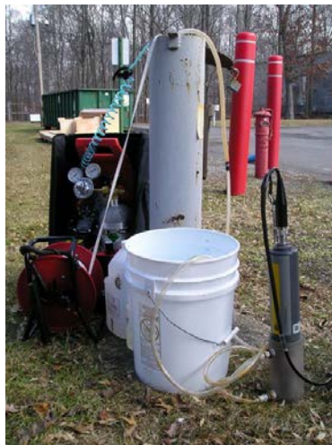
Exhibit 6-5. Well Monitoring Set-up
