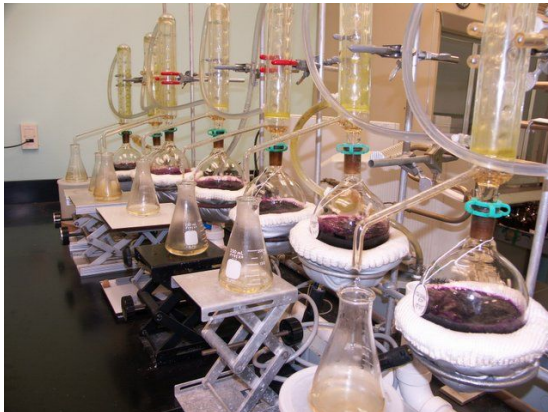
Exhibit 7-2. Distilling Samples for Tritium Analysis Performed at PEARL
