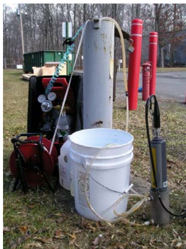
Exhibit 6-5. Well Monitoring Set-up
