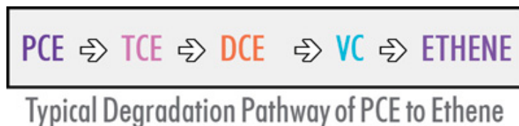
Exhibit 6-7: Typical PCE Degradation Pathway
