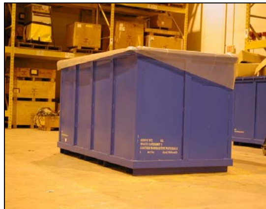
Exhibit 5-5. B-box with Liner in RWHF for Shipping Radioactive Waste
