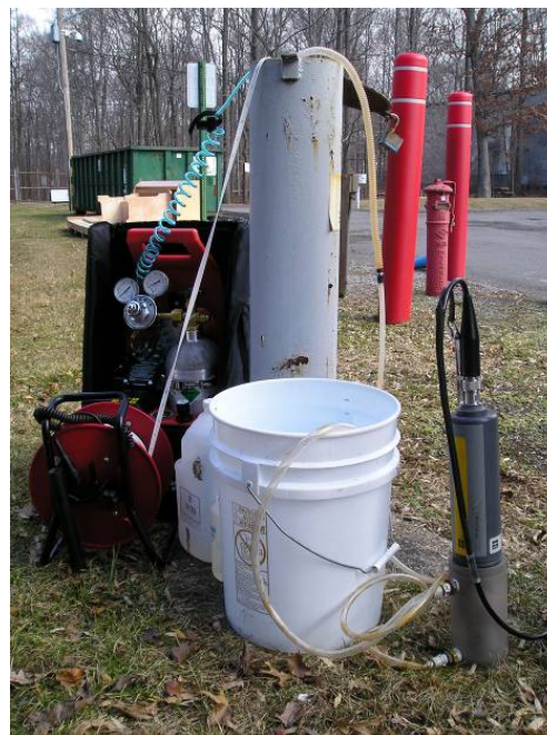
Exhibit 6-5. Well Monitoring Setup –Compressed Air, Water Depth. Meter, Discharge Collection Bucket, and Probe
